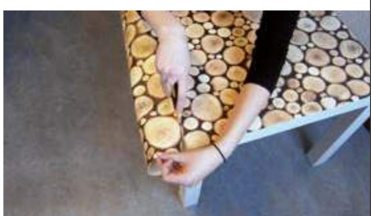
Remove excess film using a sharp knife along a ruler or straight edge and then smooth over.
